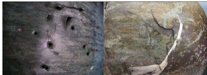
Figure 3: Holes, fissures and green corrosion product on the Spheres of the Yamur before restoration. Image: Eugenio Fernández Ruiz (IAPH)
